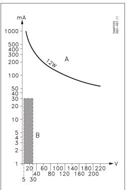
Curve A gives the maximum load. Hatched area B: Acceptable load for the gold plating of the contact.
