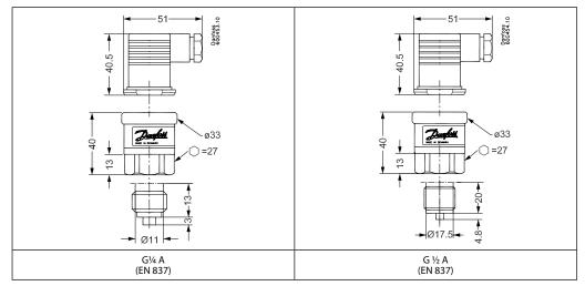
$Recommended \ torque = 30-35 \ Nm \ (Depends \ of \ different \ parameters \ as \ packing \ material, \ mating \ material, \ thread \ lubrication \ and \ pressure \ level.)$
