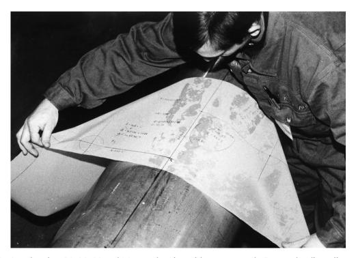
2. Punch points P1, P2, P3 and P4 onto the pipe with centre punch. Ensure that lines dissecting the points can be redrawn once the paper is removed.
