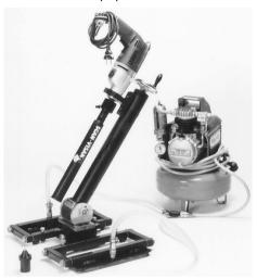
The unit contains a core drill bit, an ordinary handheld drill and a device for fastening the unit to the pipe wall.
