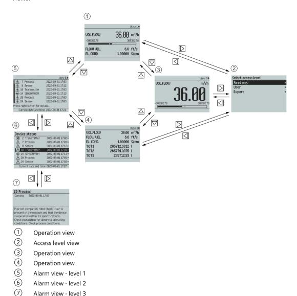
You can navigate through the menu structure items in the device using the four buttons on the display as described below.
