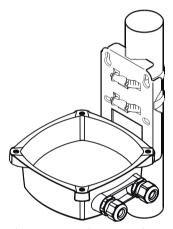
Figure 5-4 Pipe mounting - vertical
