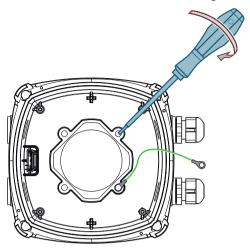
5. Rotate the terminal box and remount it on the pedestal. Make sure that the gasket is properly installed between the terminal box and the sensor pedestal.
