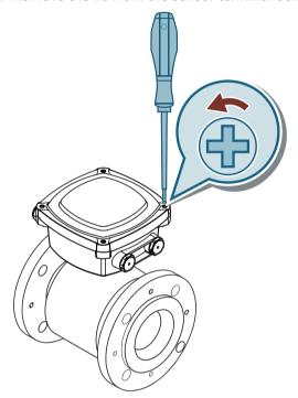
2. Remove SENSORPROM from the holder in the sensor terminal box. The SENSORPROM has to be mounted in the transmitter terminal box.
