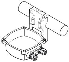
Figure 5-5 Pipe mounting - horizontal
