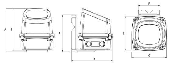
Figure 13-2 Transmitter dimensions wall mounting unit
