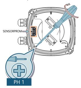
4. Fit coil and electrode cable ② through the cable glands. Connect coil cable ① and electrode cable ② in the corresponding terminals on the terminal blocks. Tighten all terminal screws with maximum torque: 0.5 Nm.
