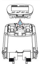
5. Connect the SITRANS AW050 Bluetooth adapter to the transmitter using the supplied flat cable.
