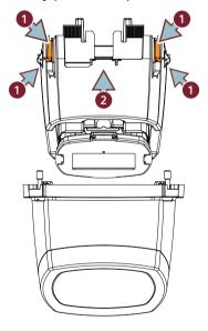
4. Lift off the display and rotate to your desired orientation.
