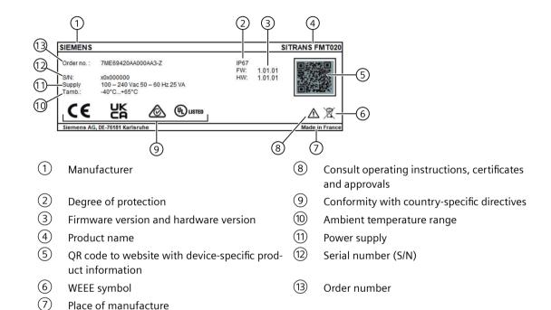
Figure 4-1 Nameplate layout, example
