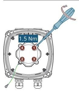
6. Remount the connection board and cables as described in Connecting the transmitter in compact design (Page 48).
