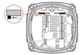
4. Mount the transmitter on the terminal box by cross tightening as indicated. To avoid damage to the device do not fully tighten right away.
