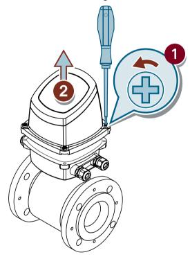
3. Unscrew all cables and remove connection board from terminal box.
