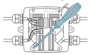
4. Unmount the terminal box from the sensor pedestal.
