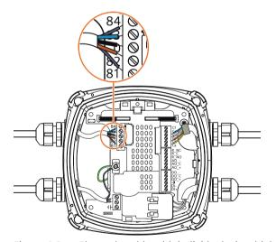
Figure 6-3 Electrode cable with individual wire shields
