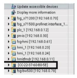
To assign the PROFINET device name to the device, select the MAC address of the device and open it online. Enter the name in the "PROFINET device name" field. This is the name that will be used to identify the device on the PROFINET network.
