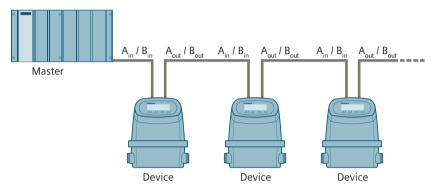
Figure B-2 Modbus connection
