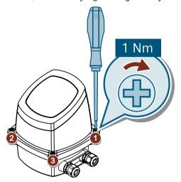
10. To obtain optimum sealing, tighten cable glands.
