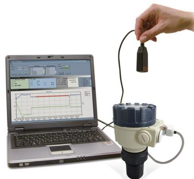
The IrDA adapter and the IrDA port of the device must be placed within a 5...10 cm distance and facing each other!
