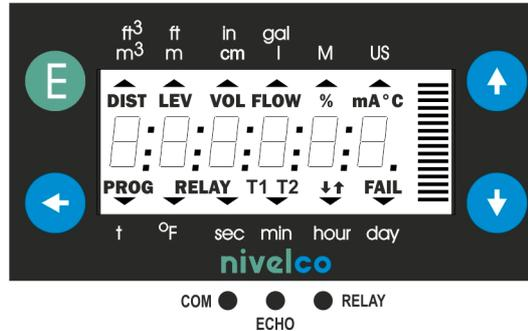
By holding the **↑** (UP) arrow button the display shows the transducer (also the air inside the tank) temperature.
