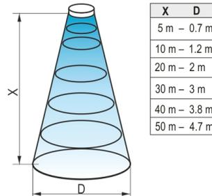
Diameters corresponding to the  $5^\circ$  beam angle.
