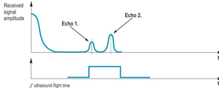
Some applications involve multiple (target + interference) echoes even within the measuring window. The Quest program will select the echoes automatically. This parameter only influences selecting the echo in the measuring window.
