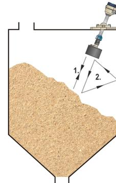
If this parameter has been used (P33 ≠ 0), its value will be continuously updated with the correct echo position. It means that in case of a power loss, the EchoTREK will restart the signal processing with the measuring window at the last updated position. To switch off this function, set P33= 0.
