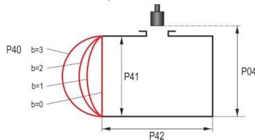
Standing cylindrical tank/silo with conical bottom a = 1, b = 0
