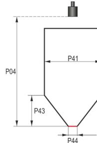
Standing rectangular tank/silo with or without chute a = 2, b = 0
