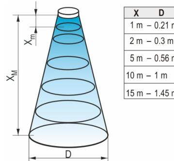
Diameters at 5° beam angle.
