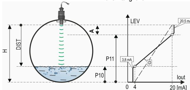
**A:** Shortest measurable distance**D:** diagram valid for default values of **P10** and **P11**
