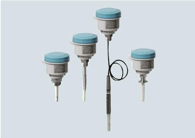
Pointek CLS200 (standard version) is a versatile inverse frequency shift capacitance level and material detection switch with optional rod/cable choices and configurable output. CLS200 is ideal for detection of liquids, solids, slurries, foam, and interfaces and has the ability to tune out buildup on the probe.
