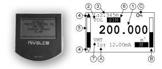
**A.**, Calculated value of the output current. After the dimension, the mode of current output is indicated by inverse inscription:
