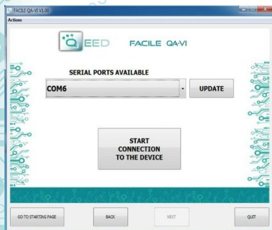
It is possible to use the program without connecting to the module, in this mode you can SAVE the configuration on your PC, which can then be sent to the QA-VI at a later time.
