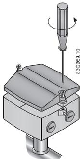
2. Mount the two terminal blocks as shown and insert electrode cable plug ① (terminals 82, 0 and 83) and coil cable plug ② (terminals 85 and 86).
