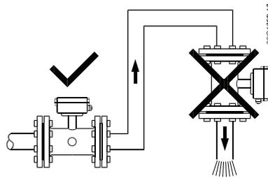
Figure 4-4 Correct installation at low point before outlet
