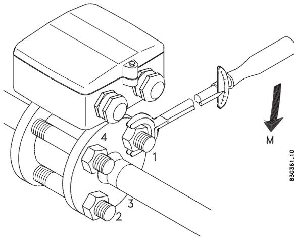
The bolts must be tightened using up to 50% of the max. tightening torque for the pipe dimensions stated. The max. tightening torque for different size pipes is given in the table. The bolts must now be cross-tightened in the sequence shown, using up to 100% torque.
