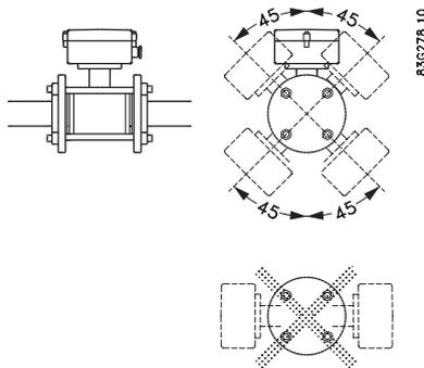
Figure 4-6 Horizontal installation, various terminal box positions
