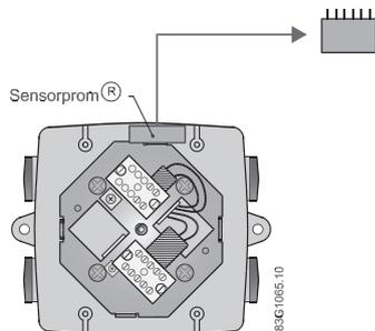
4. Fit the ½" NPT or M20 cable glands for supply and output cables.
