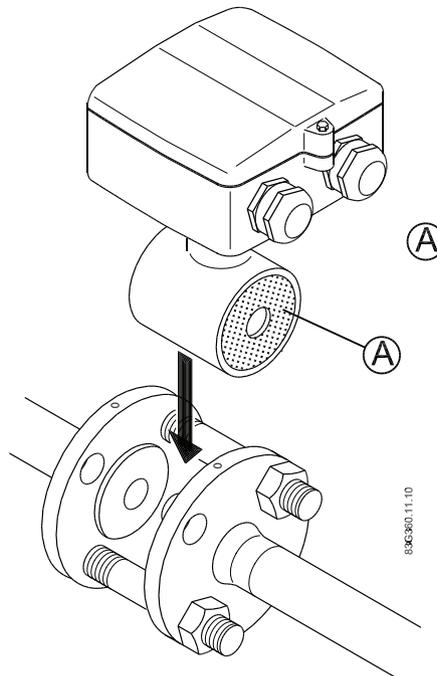
The remaining flange bolts can now be inserted and tightened using about 25% of the actual tightening torque, see table below.
